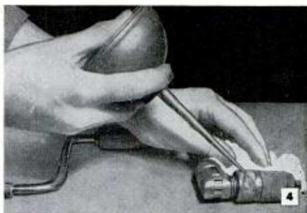
Light machine oil applied to exposed metal surfaces is always reliable as a rust preventive on hand tools
